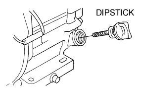
Figure 6. Engine Oil Dipstick Removal
